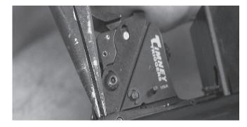
7) Before installing the action into the stock, inspect how the trigger fits the opening on the trigger guard. The trigger guard may need enlargement to accommodate the wider Timney trigger shoe. Some stock inletting may also be needed.
