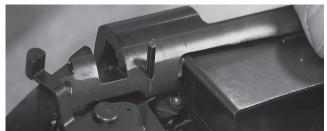
5) Tap the rear pin from left to right until it is flush with the bolt release.
