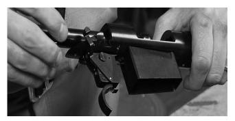
9) With an empty chamber or with Snap Caps installed, with the safety lever on Safe, pull the trigger. The firing pin should not move.
