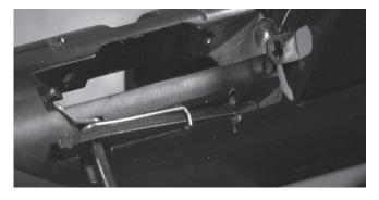
6) Adjust the bolt release so it moves the bolt stop without any binding. Do this by very slightly bending the tip with needlenose pliers so it perfectly engages the notch in the bolt stop. Bend and test.
