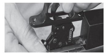
8) Install the bolt in the barreled action and check trigger function and safety function.
